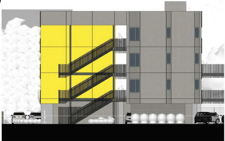
BUILDING B2 WEST ELEVATION 1/8" = 1'-0"
