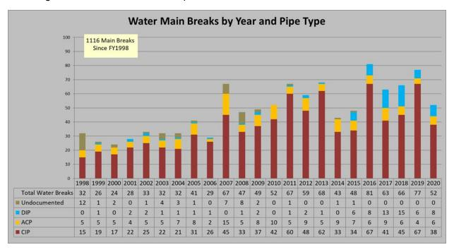
Water main breaks throughout the City are mapped and this information is used to determine the locations of waterline replacement projects. The table and map on the next page show the projects completed to date and planned projects through 2027.
