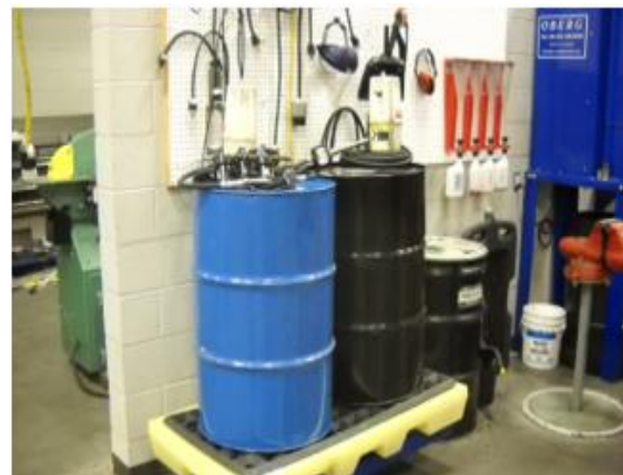
Secondary Containment for pollution control
