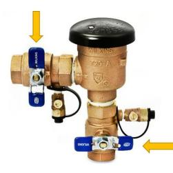
This is what a general back flow preventer looks like. This one specifically is a pressure vacuum breaker which has two ball valves: one right before and right after the breaker. These count as your irrigation shut off valves.
