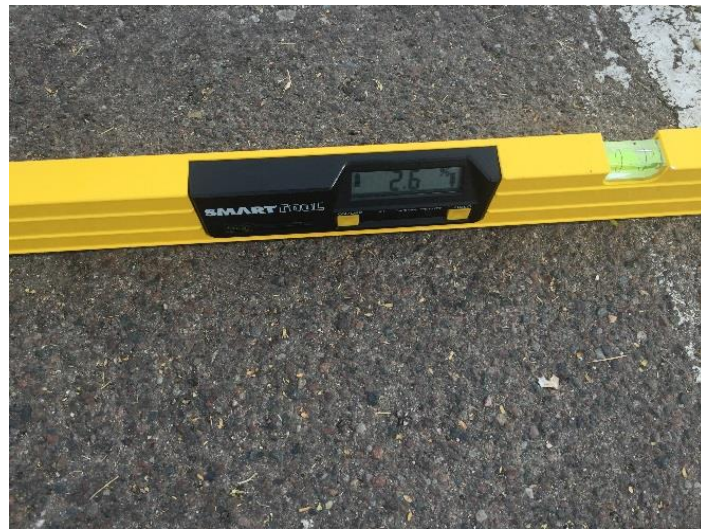
Figures 19 and 20: Slopes greater than 1:48 within accessible parking
