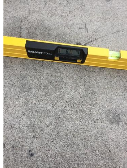
Figures 8 and 9: E. 7 th St. – Slopes up to 6.0% within parking spaces
