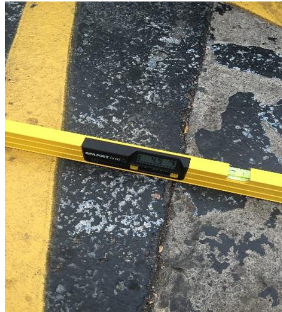
Figures 10 and 11: W. 4 th St. – 4.9% slope within parking spaces
