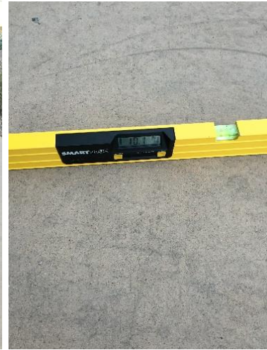
Figures 25 and 26: Curb ramp slope 10.9%
