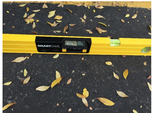
Figures 15 and 16: City Hall West – 4.0% slope within space and aisle
