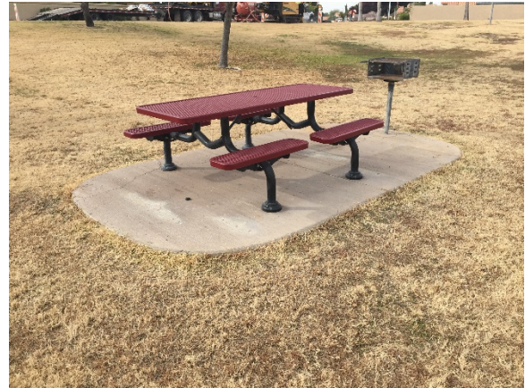
Figure 28: Corbell – Ex: No accessible route to amenities
