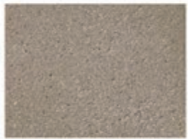
INTEGRAL COLORED CONCRETE FINISH: SANDBLAST
