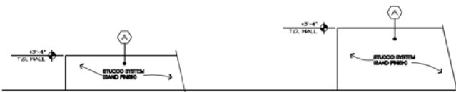
PARKING SCREEN WALL SITE WALL ELEVATIONS
