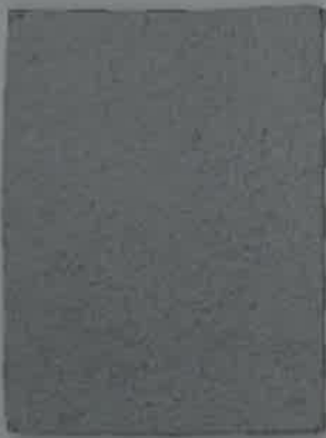
EXTERIOR INSULATED FINISH SYSTEM (EIFS-01) MANUFACTURER: DRYVIT COLOR: THUNDERCLOUD GRAY 2124-40 TEXTURE: FREESTYLE
