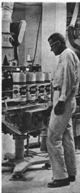
Carl Hammond, head packer at the Hayden Flour Mills, checks equipment weighing each bag of Rose Flour, adding just the right amount to bring the weight to five pounds. The bags are then automatically sealed and packed for shipping.
