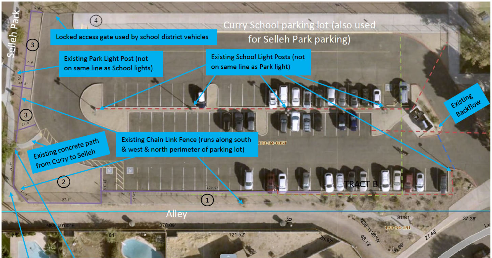
Figure 2. Aerial with Measurements and Object Identification (Chain-link fence posts are ~10ft apart)
