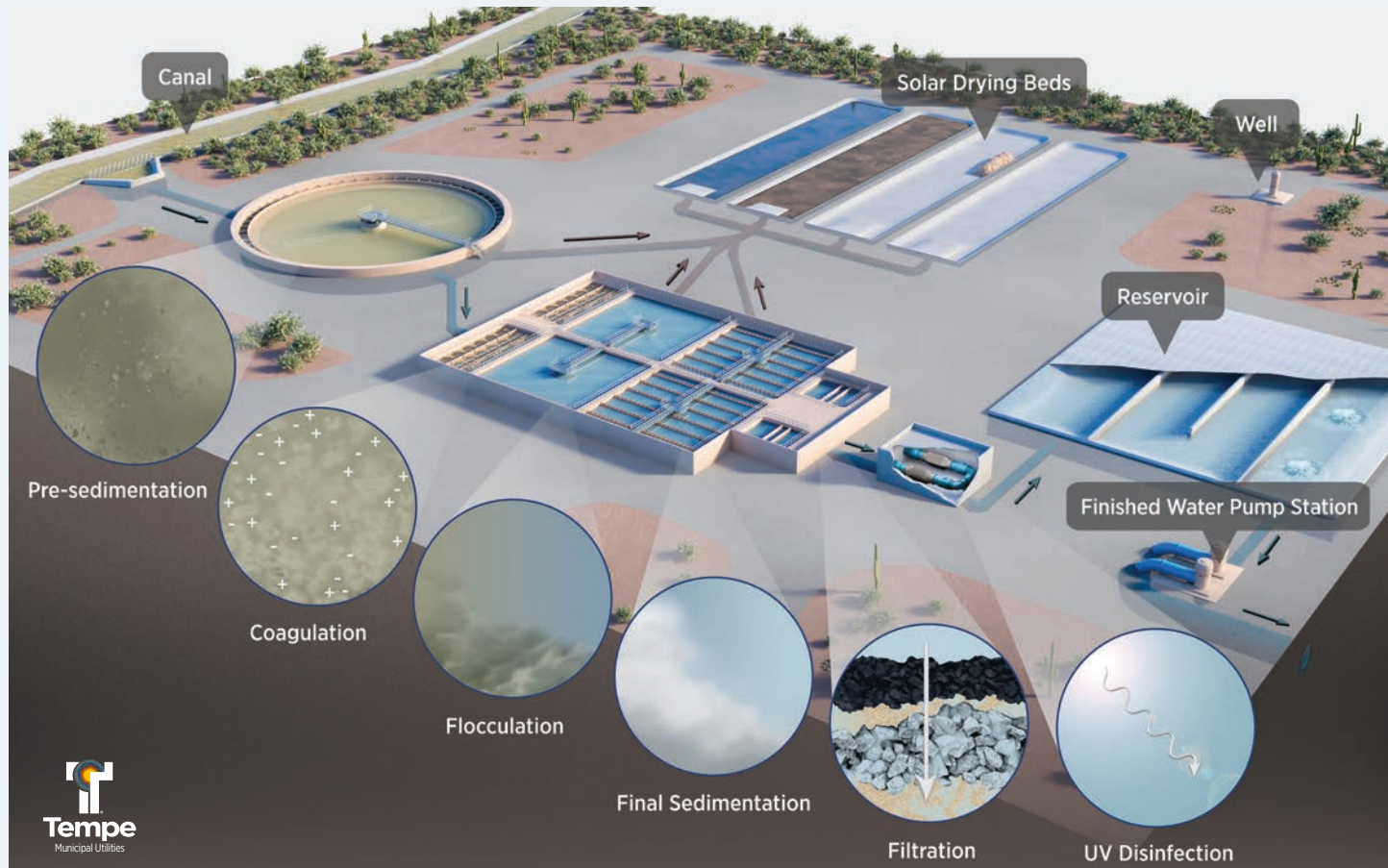
Figure 1: The surface water treatment process involves removing solids, disinfecting and purifying water that enters the plants from wells and canals. Visit tempe.gov/operations to explore the process.
