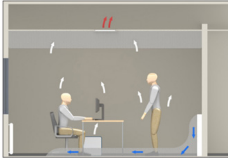
Stratified Room Air Distribution (source: Titus HVAC)
