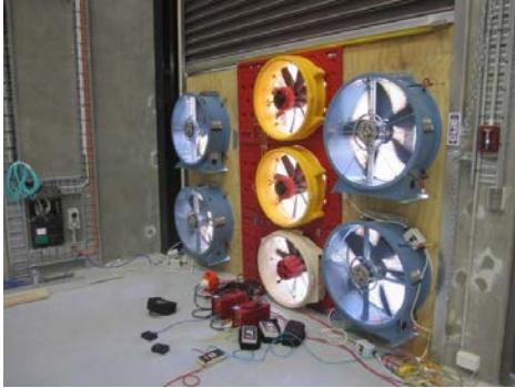
Example of a Blower Door Test equipment
