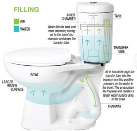
Niagara UHET - Filling Mechanis
