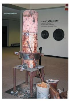
of the metal. (He was buried in an iron casket.) In 1794 he was granted a patent to produce iron for cannon, using the invention he called a cupola furnace. Its meaning today has narrowed to a furnace for iron re-melting in the foundry. Such devices are economical and extremely productive.
