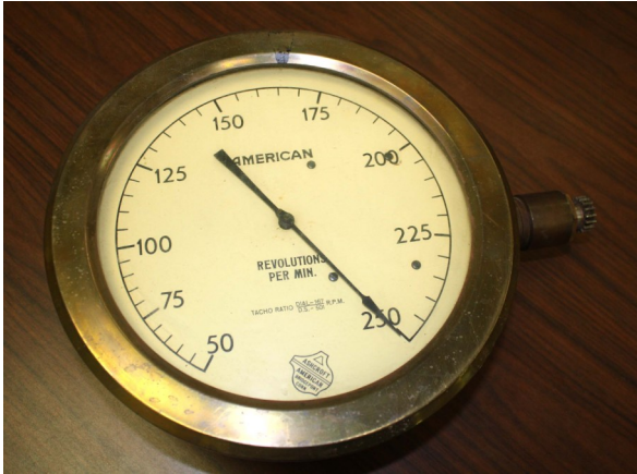
1937 tachometer from the generator at the SRP Crosscut Steam Plant in Tempe. Donated by Donald Squire.
